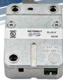
Like the Universal, this innovative design offers 8-way flexibility in installation, but fits the industry standard "Magic Module." The EM20 may be mounted either RH, LH, VU or VD or it may be flipped over to block a reversed boltwork design. Ships standard with our Basic board (EM20•20), but may be ordered with a DIA (EM20•50), DIA Pro (EM20•55) or Digital board (EM20•60).
